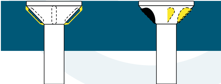
6 Vertical lobes enlarge the hole around the CSK Head. Comes loose when shaken.
